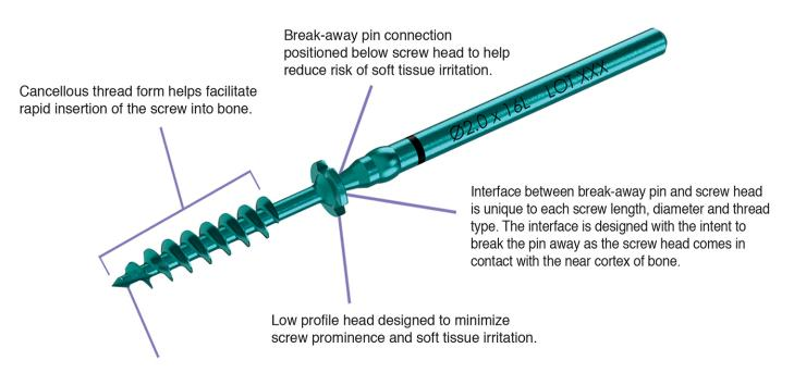
Self-drilling and self-tapping screw tip allows for screw insertion without a pilot hole.
