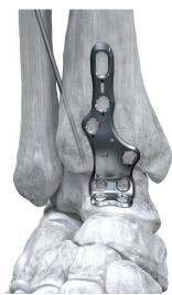
Frequently there is an irregular surface remaining over the anterior joint which requires debridement to a smooth surface with either a rongeur or saw. Retrieve the appropriate anterior TT plate based on the patient's anatomy. To position the plate, palpate the medial and lateral margins of the talus and center the talar portion of the plate. Ensure that the proximal plate is midline or just lateral to midline.
