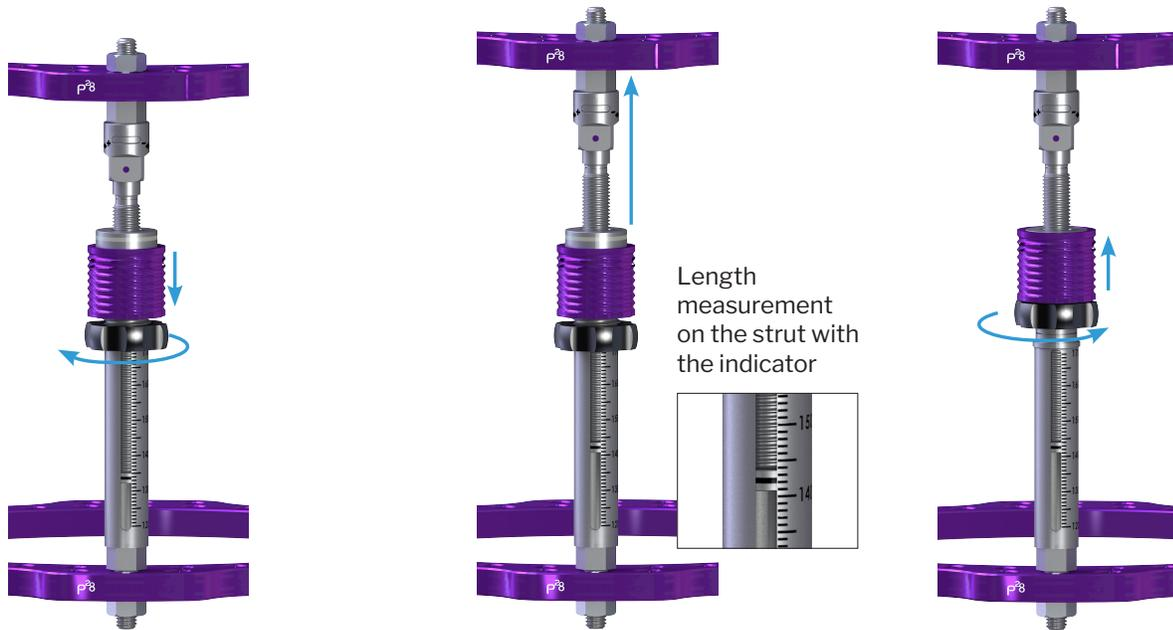
Length measurement on the strut with the indicator
