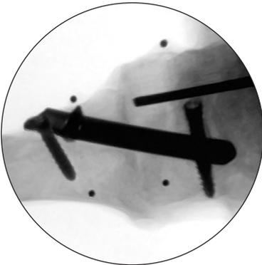
Figure 2. A Phantom® Intramedullary Nail undergoing in vitro cyclic testing.
