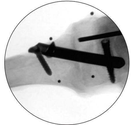
Figure 5. Phantom<sup>®</sup> Intramedullary Nail showing 0.3 mm of plantar gapping after 20,000 cycles.
