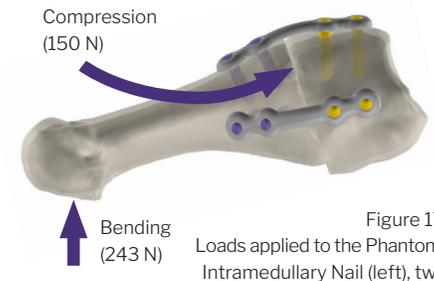
Figure 17. Loads applied to the Phantom® Intramedullary Nail (left), two crossing screws (middle), and biplanar plates (right).
