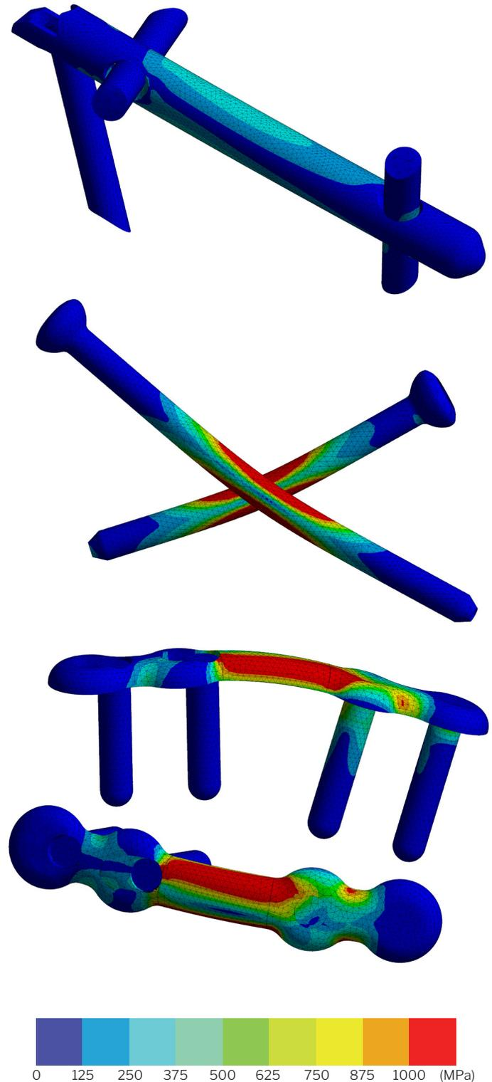
Figure 11. Implant stress for the Phantom® Intramedullary Nail (top), two crossing screws (middle), and biplanar plating (bottom) for the 2 mm initial gap scenario.
